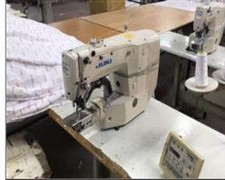
Photo of non-conformity NC bartak machines were found not equipped with safety eye glass.jpg
